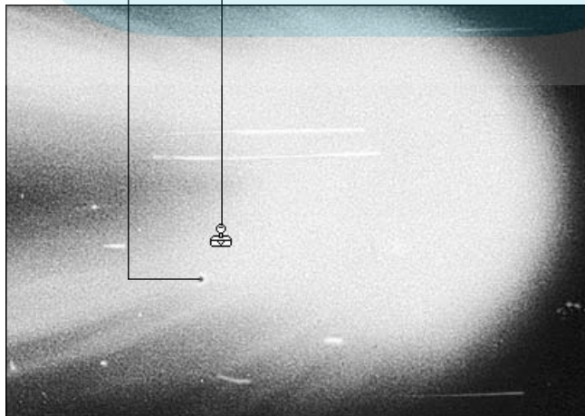
Figure 11-5: Alt+click (Option+ click on the Mac) on a good portion of an image to establish the cloning source.
